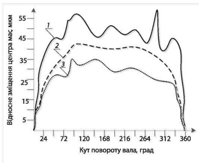
Fig. 4. Results of mathematic modeling of relevant displacement of centre of masses of the bearing of the degree of rotation of the shaft at the frequency of rotation 1000 rev/min and loading 1500 H: 1 – traditional slide bearing with the lubricant fluid; 2 – developed hydrostatic slide bearing, lubricant fluid-hydro-layer; 3- developed magnetic slide bearing, lubricant fluid – magnetic lubricant
