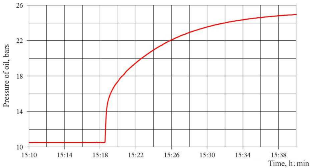
Figure 8 – Change of oil pressure over time at the distance of 19 km from OPS 2 when starting a pumping unit based on experimental results (oil flow before starting was 1140 m 3 /h)
