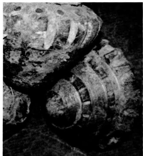
Figure 2 – Abrasive wear of three-cone bit from 14HT3MA-B steel
