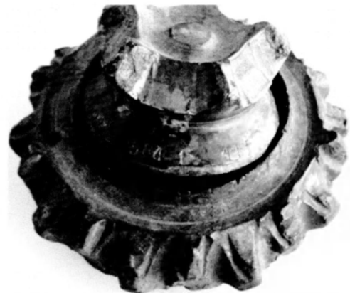
Figure 1 – Fragile fracture of the cone from 14HT3MA-B steel
