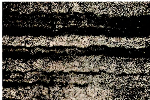
Figure 9 – Inappropriate structural heterogeneity in the form of coarse striping on one of the steel melts 14HN3MA (roll stock in the state of delivery) × 100
