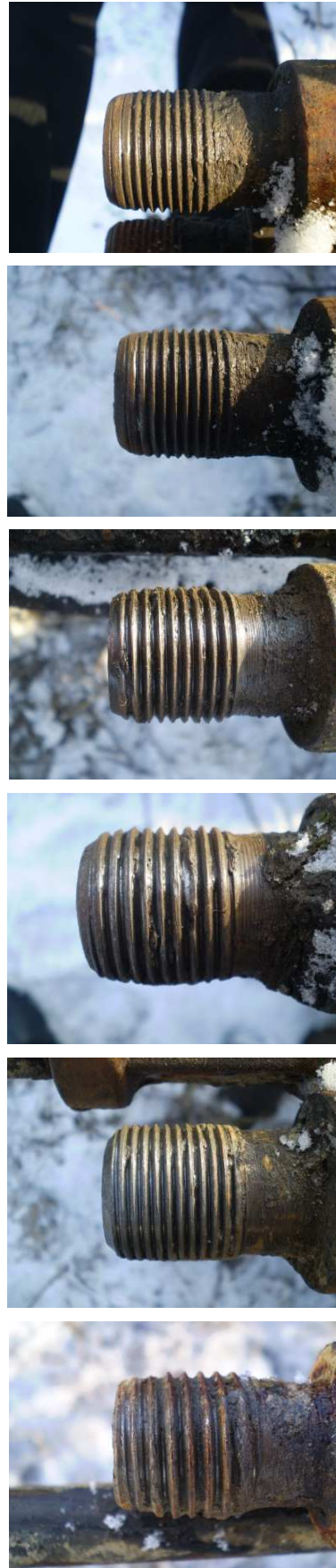
Figure 6 – Worn sucker rod thread
